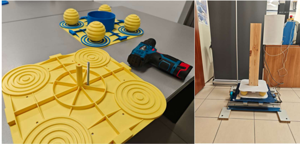
Figure 10- Small scale experiments of Type-B isolators.
